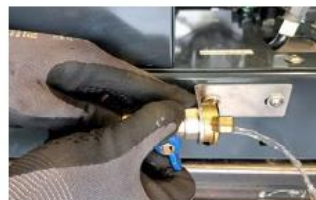
STEP 4 Empty the water tank to avoid algae formation
