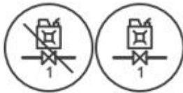
Dieselventil 1 OFF / Dieselventil 1 ON
