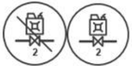
Dieselventil 2 OFF / Dieselventil 2 ON
